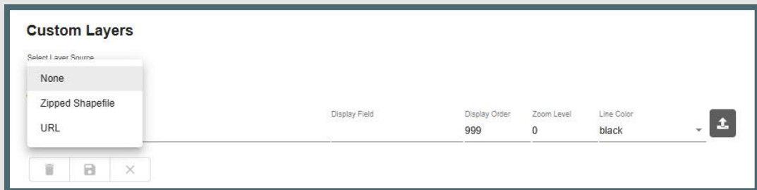
Figure 10 - Select either a zipped shapefile or a URL to add a custom data layer.
