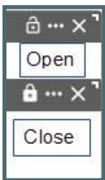
Figure 170 - The Freeze Lock in the “Open” position allows the panel to move. The “Close” position docks the panel in place on the Home page.
